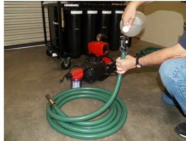
Fill hose with water
